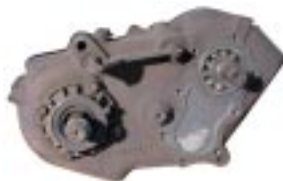
NP205 T/C figure-8 bolt pattern
