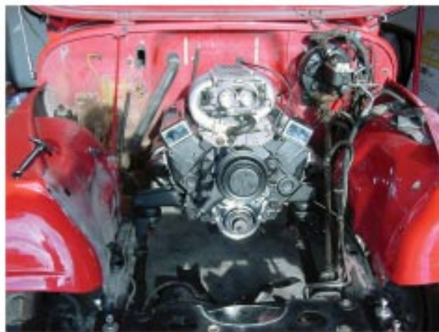
713089 bolt-in mounts with engine off-set
